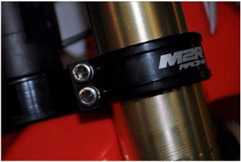
Check your head set has no play in it tighten if required. Don't over tighten this as you could crush the head set bearings, or make the steering hard to turn.
